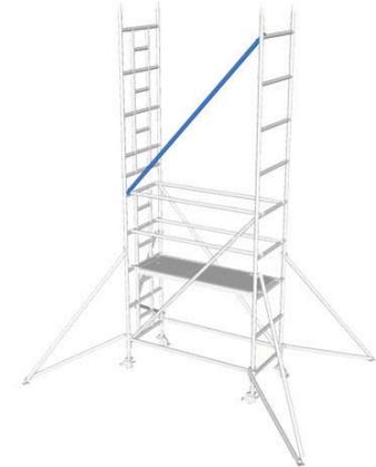
6. Fit one long diagonal brace as close to one of the frame vertical tubes as possible.
