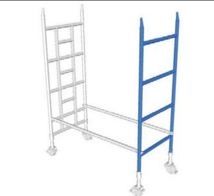
3. Fit opposite ends of short braces to other 4 rung frame ensuring pegs on frame head fitting point towards middle of tower.
