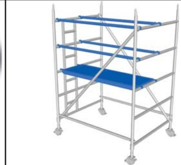
3. Fit 2 long braces diagonally in opposite directions as close to the vertical tube as possible. Fit a temporary platform on the 3rd rung down from the top of the frame &, working through the trap fit short braces as temporary guardrails horizontally onto top & 2nd rung of frames between pegs provided. Level the tower by adjusting collar on castors (see construction notes)
