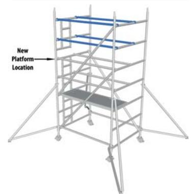
9. Fit short braces on the top 2 sets of rungs to form guardrails as before. Remove the current temporary platform & relocate onto 5th rung of the base frame.
