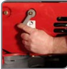
Simple lever from single to dual flow at the front of the cab.
