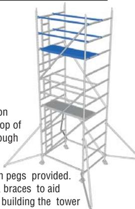
11. Fit a trap platform on third rung down from top of frame and working through trap fit short braces horizontally on top rungs of frame between pegs provided. Still using a platform & braces to aid safe erection, continue building the tower repeating the bracing pattern until the required platform height is reached.
