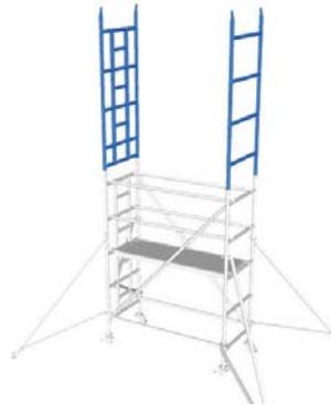
5. Working from a platform add a 4 rung ladder frame to the 5 rung ladder frame by locating onto head fitting with peg engaging into hole provided. Repeat the process at the other end using a 4 rung main frame.
