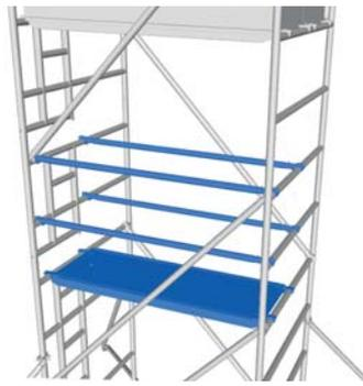
Rest platforms must be fitted every 2m and consist of a trap platform and guardrails at 1m above and 0.5m as shown. Remember to always close trapdoor immediately after climbing through.
