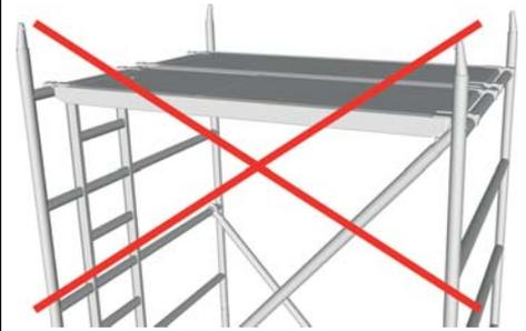
**WARNING:** never work from or build, or dismantle the tower from an unguarded platform
