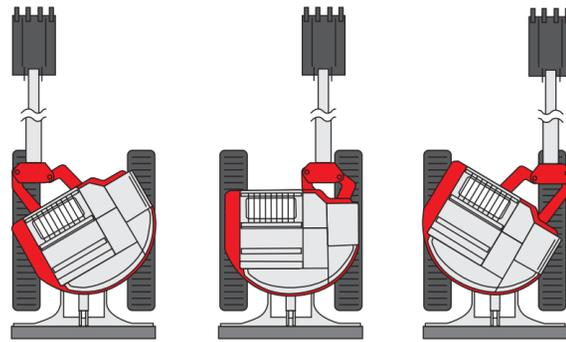
Takeuchi introduced the FR series of reduced tail swing excavators to meet the growing demands for compact operation especially where restricted access limits the size of the machine.
