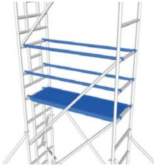
Rest platforms must be fitted every 2m and consist of a trap platform and guardrails at 0.5m and 1m as shown. Remember to always close trapdoor immediately after climbing through.
