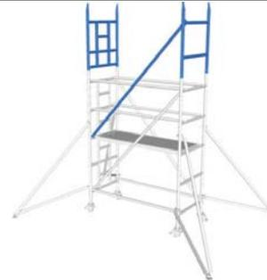
8. Work from temporary platform, add a 2 rung ladder frame to the 5 rung ladder frame by locating onto head fitting with peg, engaging into hole provided. Repeat the process at the other end using a 2 rung frame. Add a diagonal brace to the top rung of the 2 rung frame on one side of the tower.
