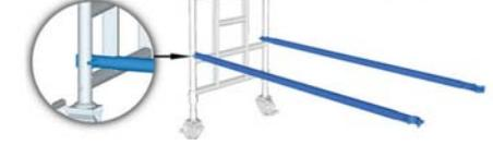
2. Make sure pegs on frame head fitting always point towards middle of tower (see detail 2B). Fit two short horizontal braces to vertical tubes of one of the frames ensuring spring loaded pin faces outwards (see detail 2A).
