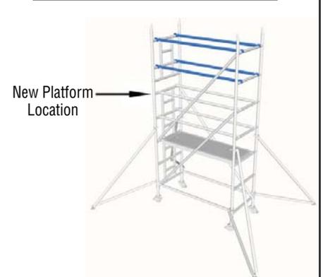
9. Fit short braces on the top 2 sets of rungs to form guardrails as before. Remove the current temporary platform and relocate onto 5th rung of base frame.
