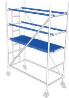
3. 1) Fit two long braces diagonally in opposite directions as close to the frame vertical tube as possible. 2) Fit a temporary platform on the 3rd rung down from the top &, working through the trap, fit short braces as temporary handrails onto frame uprights above top rungs of frames. At this stage level the tower by adjusting collar on castors (see notes).
