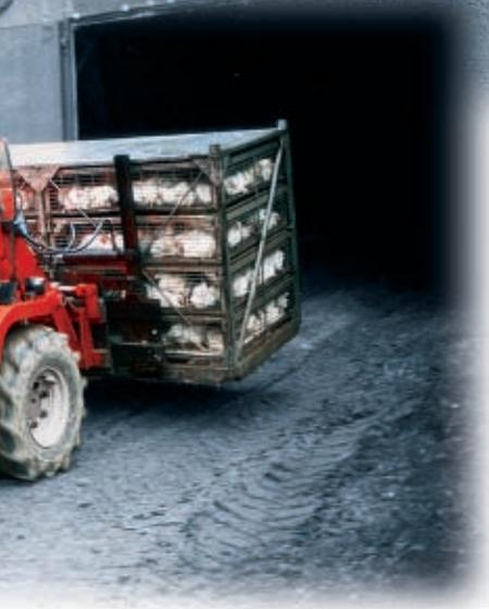
A 51 hp engine and four-wheel drive make the Buggiscope ideally suited to rough-terrain operations.
