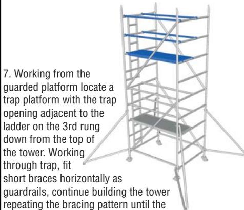
7. Working from the guarded platform locate a trap platform with the trap opening adjacent to the ladder on the 3rd rung down from the top of the tower. Working through trap, fit short braces horizontally as guardrails, continue building the tower repeating the bracing pattern until the required platform height is reached. Continue onto box 12, 13 or 14 (whichever is applicable)
