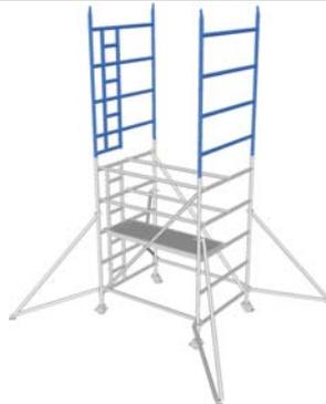
5. Working from platform add a 4 rung ladder frame to the 5 rung ladder frame by locating onto head fitting with peg engaging into hole provided. Repeat the process at the other end using a 4 rung main frame.
