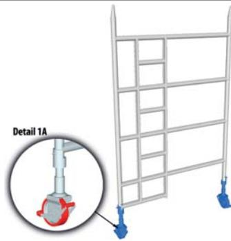
1. These towers should be erected by at least 2 competent persons. Apply brakes and fit adjustable castors into one 4 rung ladder frame and one 4 rung main frame, ensuring that spring loaded pin is engaged in hole provided (see detail 1A).
