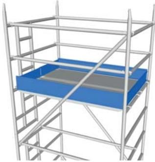
Fit the final platform ensuring that the trapdoor is above the ladder & the main (plain) platform is next to it. Fit toeboard unit around the platforms & push the 2 pins that are located at each end down. Remember to always close trapdoor immediately after climbing through.
