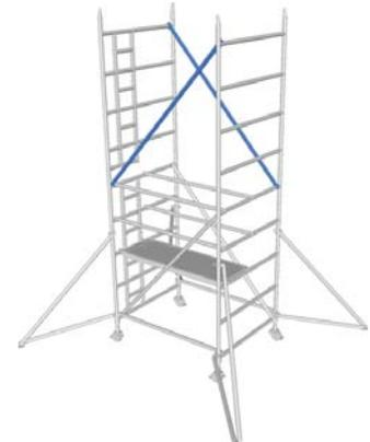
6. Fit two braces diagonally in opposite directions as close to the frame vertical tubes as possible.
