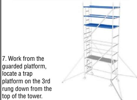
7. Work from the guarded platform, locate a trap platform on the 3rd rung down from the top of the tower. Work through it's trap, fit short braces horizontally as guard rails. Continue building the tower repeating method from 5 until the required platform height is reached, then onto box 12, 13 or 14 whichever is applicable
